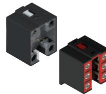
Contact blocks with captive screws, finger protection, twin bridge contacts and double interruption for higher contact reliability. They are available in multiple variants with shifted activation travels, simultaneous or overlapping. They are suitable for many different applications.
