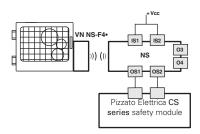
NS series switches can be used as individual devices provided that the safety outputs be evaluated by a Pizzato Elettrica safety module (see table for combinable safety modules).
