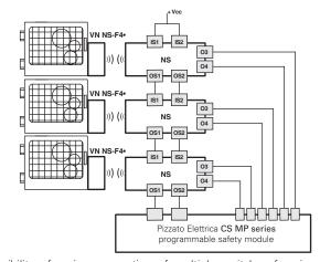
Possibility of series connection of multiple switches for simplifying the wiring of the safety system, whereby only the outputs of the last switch are evaluated by a Pizzato Elettrica safety module of the CS MP series. Both the safety-relevant evaluation and the evaluation of the signalling outputs are performed by the CS MP series.
