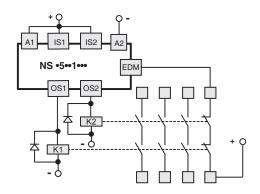
The NS •5••1••• version, in addition to maintaining the operating and safety characteristics of the NS series, allows control of **forcibly guided NC contacts of contactors or relays** controlled by the safety outputs of the switch itself. As an alternative to the relays or contactors you can use Pizzato Elettrica expansion modules CS ME-03 (see page 299). This check is carried out via the EDM input (External Device Monitoring as defined in EN 61496-1) of the switch.
