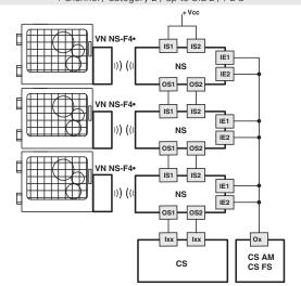
Monitoring function: actuator locked 2 channels / Category 4 / up to SIL 3 / PL e
