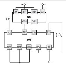
Connections with CS AR-05 •••• / CS AR-06 ••• safety modules
