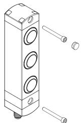
Each control device unit of the BN series is supplied complete with snap-on protection caps to be applied on the holes of the fixing screws. Not only do the caps prevent deposits of dirt from accumulating and simplify cleaning, they also prevent access to the fixing screws of the device, thereby offering increased protection against tampering.
