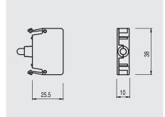
LED units for base mounting with screw connection, push-in spring-operated connection
