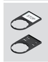
Label holders for single device, adjustable by 90° in 90° increments. The switch labels of other manufacturers can be used (for example: 3M article KE-7270-2691-3 or GRAFOPLAST article SITM612X) as long as they have the following dimensions: base 27 +0/-0.4 mm, height 18+0/-0.4 mm, thickness  $0.8\pm0.4$  mm.
