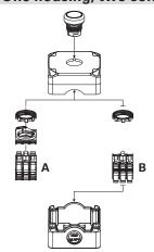
The housing can fit up to 3 contact blocks/LED units (E2 CP, E2 LP) for panel mounting by means of a mounting adapter (A) or up to 3 contact blocks/LED units (E2 CF, E2 LF) for base mounting directly on the bottom of the housing (B).
