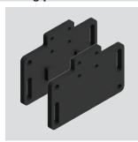
Fixing plate (complete with fastening screws) provided with long slots for adjusting the operating point. Each plate is provided with two pairs of mounting holes, one for standard switches and one for switches with reset device. The actuator thus always has the same actuating point.
