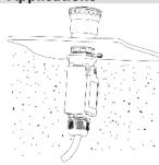
Protected contact block for control devices fitted in switching cabinets with the presence of dust also inside the cabinet. The block ensures an IP67 protection degree for internal electric contacts.
