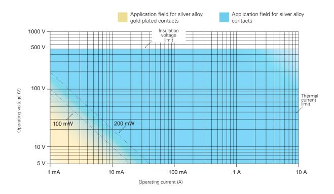
100 mW Recommended limit for general applications with snap action contact blocks with silver alloy contacts.
