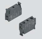
Diode blocks of the same size as contact blocks, containing a 3 A 1800 V diode inside. To be used in sections of circuits where it is necessary to ensure that the direction of current flow respects the prescribed polarity.
