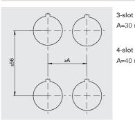
3-slot mounting adapter A=30 mm
