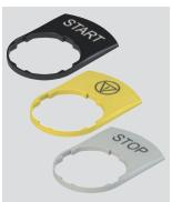
Labels for single EROUND line devices, adjustable by 90° in 90° increments. Available in black, grey, and yellow; the engraving is via laser, directly on the label itself. This avoids having to apply additional labels, and the command description remains permanent and indelible, for the entire lifetime of the label.
