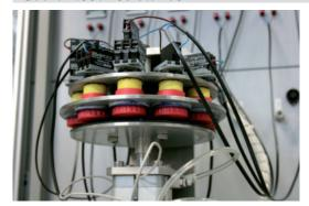
Pizzato Elettrica has tested the control and signalling devices of the EROUND line according to the specific tests of the EN 60947-5-1 standard.
