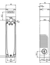
Switch FY 6 ● D5D ● Operating principle D, with key release
