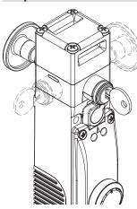
The key release device (auxiliary release) is used to permit unlocking of the actuator only by personnel in possession of the key. The device also functions with no power supply and, once actuated, prevents the guard from being locked.
