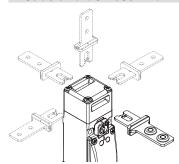
The system can be variably configured by loosening the 4 screws on the head.
