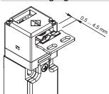
The actuation head of this switch features a wide range of travel. In this way the guard can oscillate along the direction of insertion (4 mm) without causing unwanted machine shutdowns. This wide range of travel is available in all actuators in order to ensure maximum device reliability.
