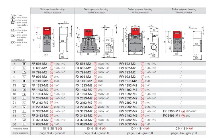
All switches listed above are available in a version with 30 N actuator extraction force. To obtain these products, the order code must be changed by adding the extension "E3", for example FR 693-M2E3.
