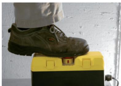
The installed devices will remain unaffected, thanks to the shape of the protection, which allows the pressure exerted to be dispersed onto the robust structure of the control station.
